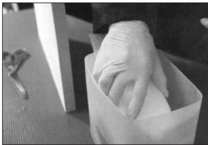
1. Pre-wet glass scrim by soaking in colloidal silica.
