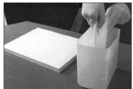
7. Pre-wet glass scrim by soaking in colloidal silica.
