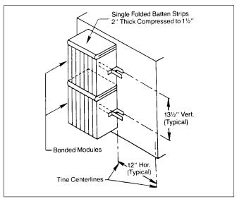
The Hefty Lock/Bonded 1800 module system is used in a wide range of applications in the temperature range up to 1000°C (1832°F). Typical applications include:
