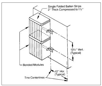
The Hefty Lock/Bonded 1800 module system is used in a wide range of applications in the temperature range up to 1000°C (1832°F). Typical applications include:
