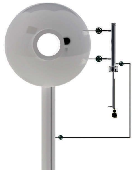
FIGURE 2 INSTALLATION DIAGRAM OF MAGNETIC LEVEL INDICATOR FOR DRUM LEVEL MEASUREMENT
